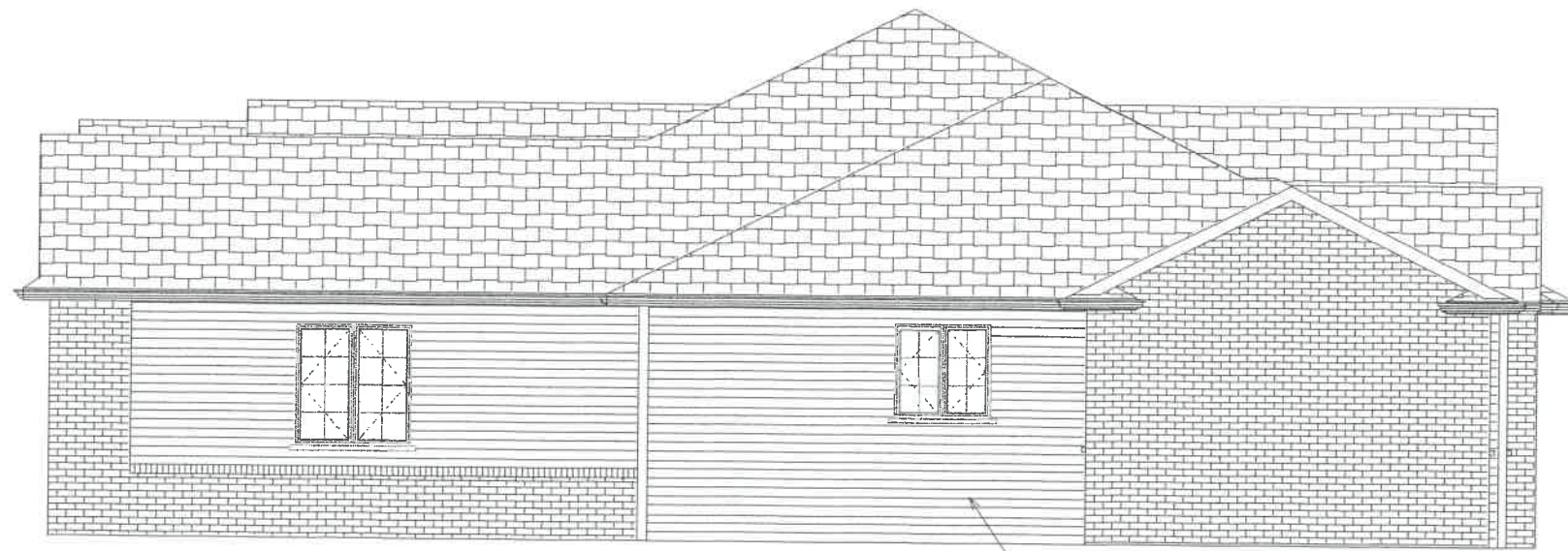
RIGHT ELEVATION 4" Vinyl Siding
